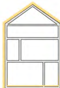
External Insulation Approach
