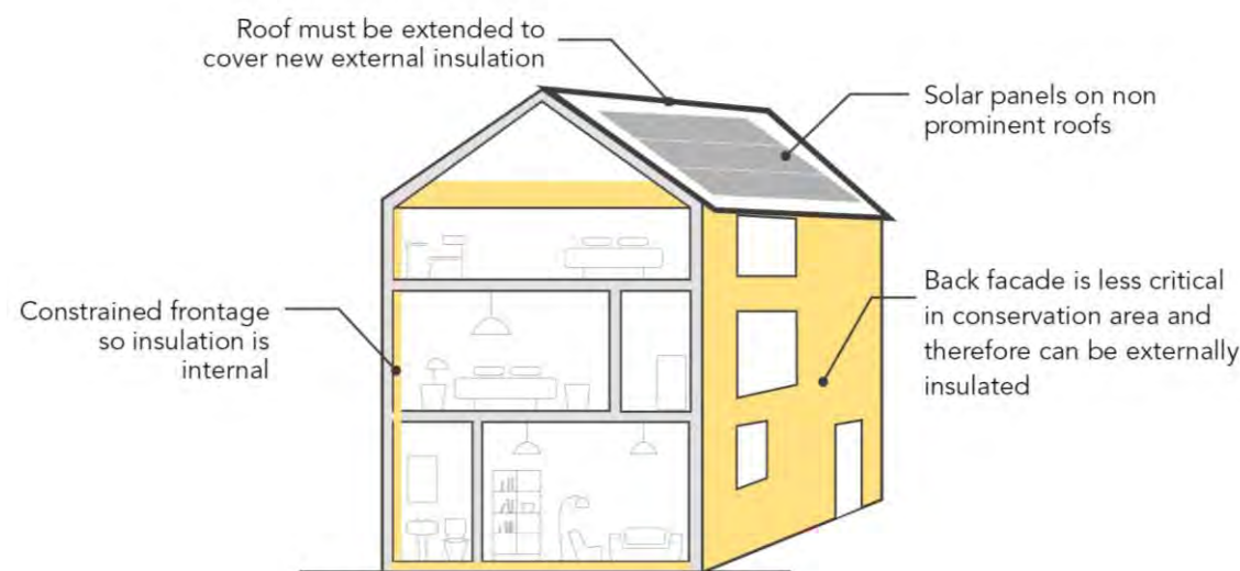
Diagram illustrating a hybrid retrofit approach with internal and external insulation.
