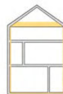
Internal Insulation Approach
